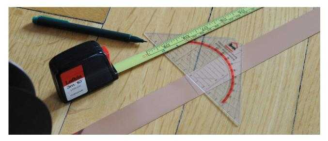
Now measure 25 mm from each end and draw a line at a right angle to mark the final length of your cable. Draw a third line at 35 mm from each end. **Mark the end of all four pieces of foil with a dot on the same side to indicate the direction.** Be careful to touch the foil only with the included cotton gloves except for the cutoff at the end.
